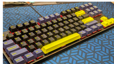
Epomaker Midnight Run "floating" over some CIY Evo Reds with 80g springs
