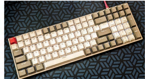
RK100 Classic version with retro PBT keys and a single bluish white backlight
