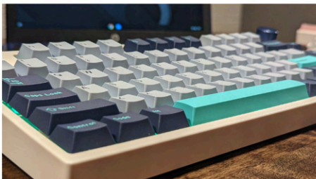
Keydous NJ80 with steel plate, Porcelain Blues switches, and a Hammerhead key clone set
