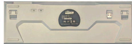
The bottom of the keyboard with switches for power and mode, dongle storage, and a pair of fold down legs.
